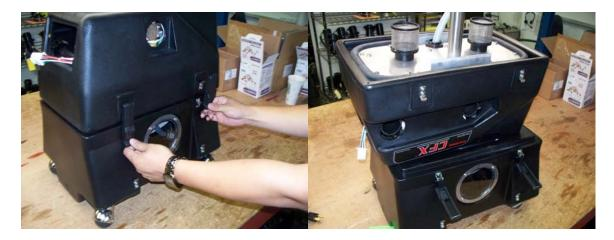
4) Use a 5/16" wrench or nut driver to remove the eight deck plate screws
