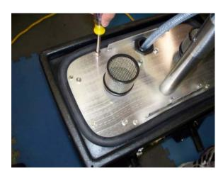
5) Holding the deck plate firmly to the top housing, turn the top housing over and place it back on top of the bottom housing.
